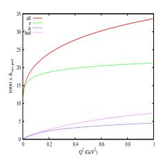
Vacuum polarization corrections due to electrons (e), muons ( $\mu$ ), hadrons (had), and the combined effect (all).
